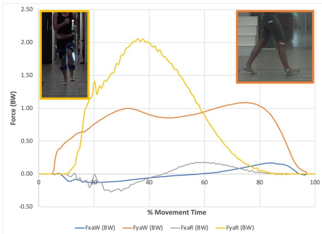
Figure 3. Lab 5: Normalized GRF profiles, walking (W) and running (R) comparison. The insets depict sample screen shots of participants' walking (orange border – sagittal view) and running (yellow border – frontal view) on the force platform.
