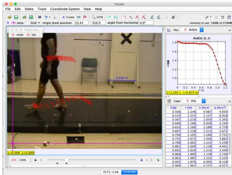
Figure 1. Screen shot of video analysis tool (Tracker) with sample processed analysis of gait cycle (Lab 2) video.
