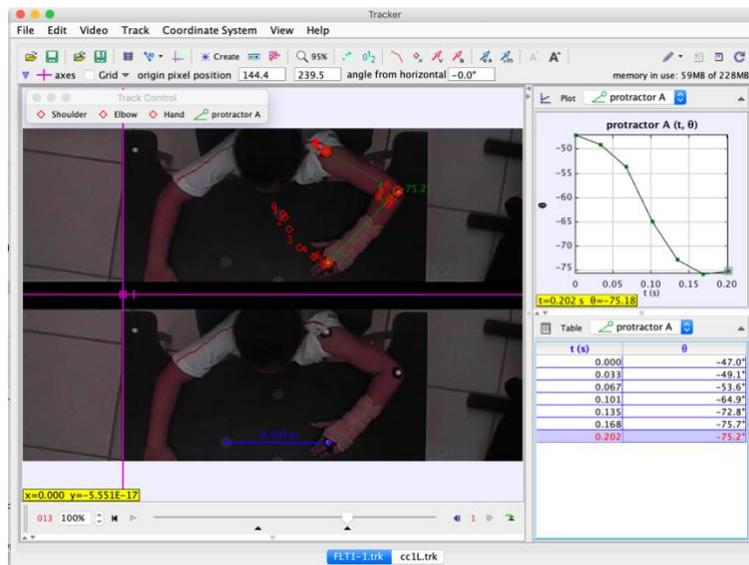
Figure 2. Screen shot of video analysis tool (Tracker) with sample processed analysis of reaching task (Lab 3) video.
