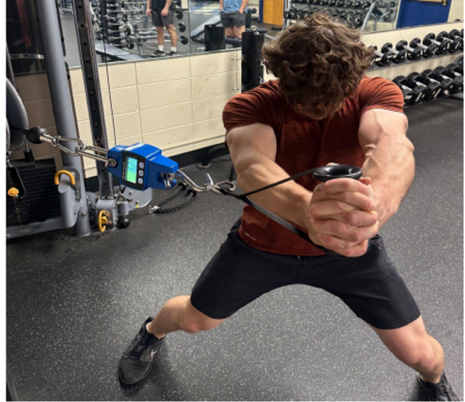
Figure 2: Isometric Core Rotation Test Set-Up.
